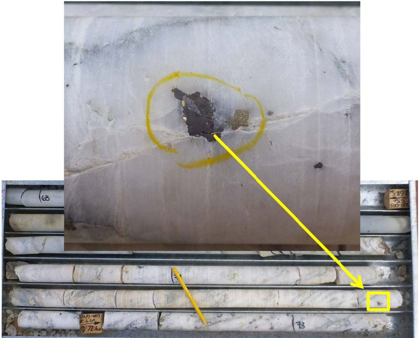
Figure 4: Black Flag West – Visible gold in drill hole BUD003
