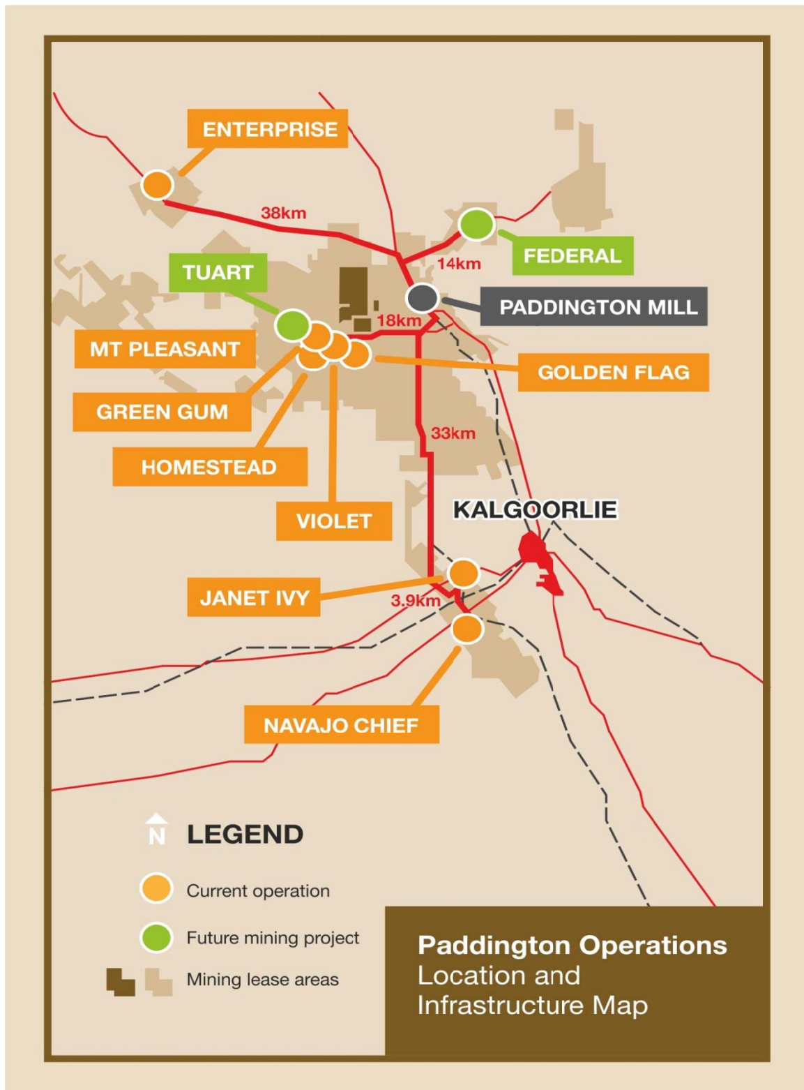
Paddington Operations location map: Paddington mine sites and haul distances to the plant.
